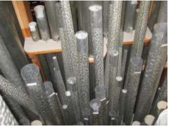
When finished, the repaired and cleaned pipes will be reinstalled, along with the new racks. The remaining pipes will then be re-installed. As the pipes are put back into the organ, the instrument will be re-voiced, regulated, and thoroughly tuned. The congregation will undoubtedly notice a significant improvement to the organ after its restoration!
